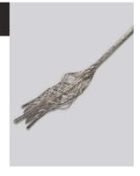
Remove the earth braid leaving approximately 10mm of braid exposed covering the heater cores.
