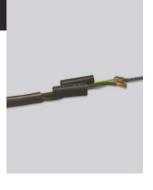
Ensuring the solder sleeve covers the earth connection use a heat gun to shrink the solder sleeve.
