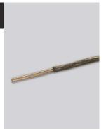
Using wire strippers strip back approximately 7mm of the insulation from the heater cores.
