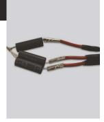
Slide the small heat shrink pieces over the butt crimps so that the entire crimp is covered. Use a heat gun in order to activate the heat shrink.
